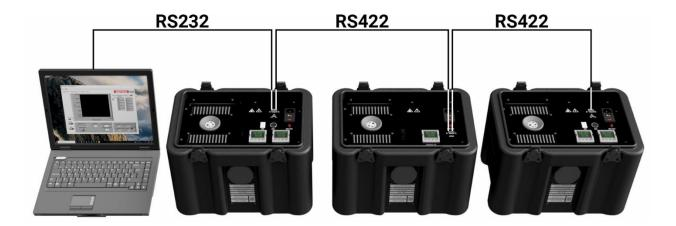
Note: The RS 422 standard specifies a maximum lead length of 1200M (4000ft). A true RS422 port will be required to realise such lead lengths. The Isotech conversion leads are suitable for maximum combined lead lengths of 10M that is adequate for most applications.
