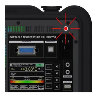
In the event that the equipment is taken into a cold environment for use, as the temperature drops you will see the red beacon illuminate. The dry block will continue to function as normal but the internal heater will continue to keep the internal components warm whilst in the cold environment.
